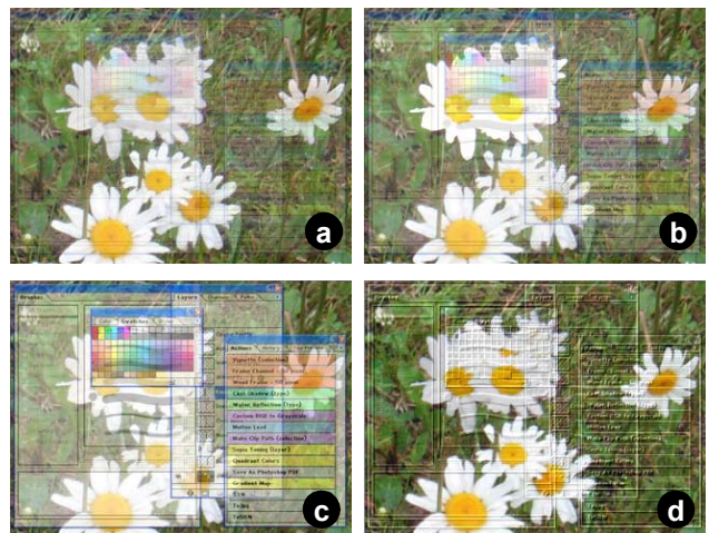
Figure 10: The 4 conditions in the background recognizability task: (a), alpha-blended at 10% opacity, (b) alpha 25%, (c) alpha 50%, and (d) glass palettes.
