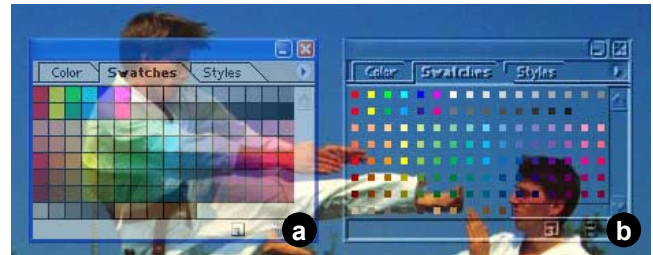
Figure 8: (a) Alpha blending dilutes colors in color palette. (b) Glass palette with manually cropped swatches (see ACM digital library for color version).
