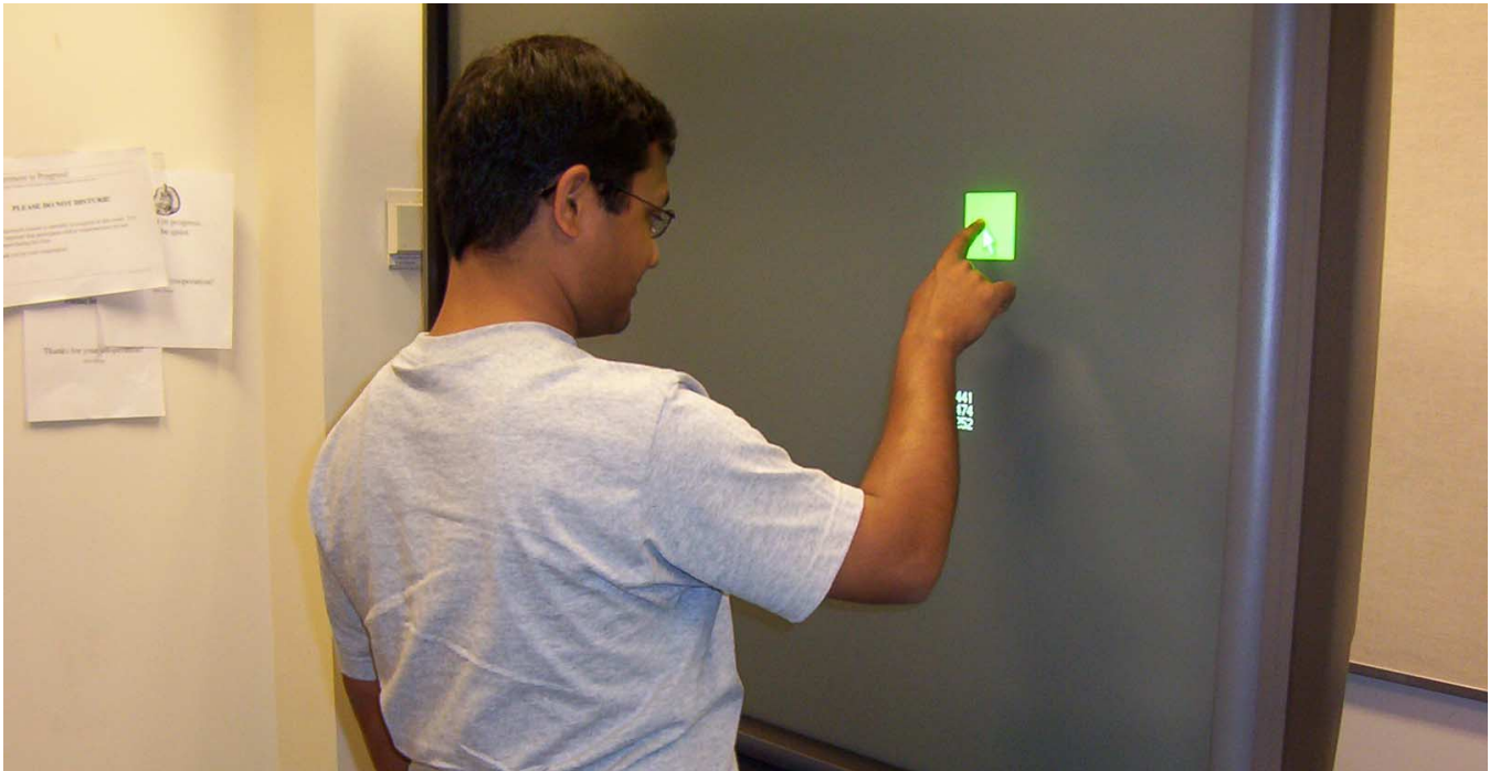
Figure 1. The SMART Board display used during the user study. Subjects stood upright during each block of trials. While fixating on a designated location on the screen, subjects either pointed directly at displayed items by touching them or indirectly by using an optical mouse (not shown). The designated location of fixation determined whether selected items appeared in the UVF or LVF.
