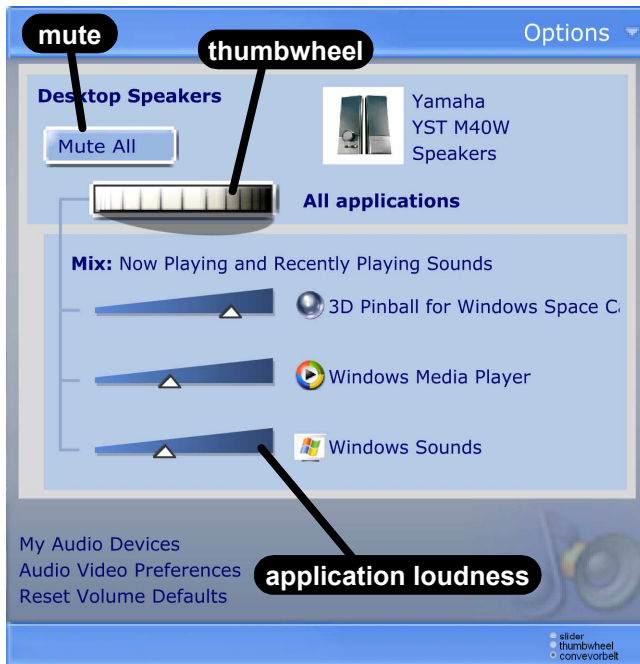
Figure 3: The flat volume control panel. Application sliders represent the loudness of that application. Thumbwheel and mute affect all application sliders.
