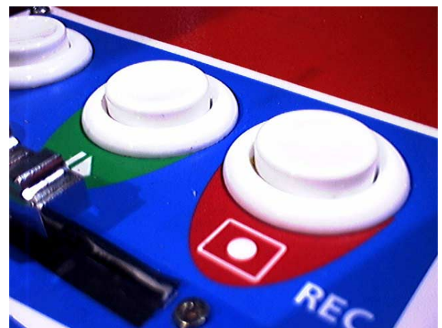
Figure 11. The panel inside the dome contains buttons for capturing and deleting frames and previewing the animation.
