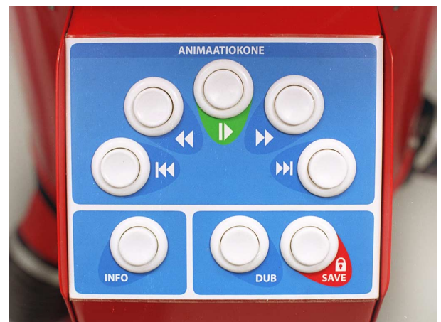
Figure 12. The buttons on the front of the machine allow browsing the animations, recording a soundtrack, saving the animation and displaying an introductory video.
