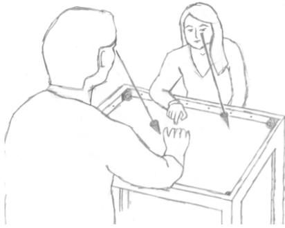
Figure 1. The envisioned GazeTop system: infrared (IR) cameras are placed at each corner of the table. IR LEDs are distributed around the perimeters of the table and act as point light sources. Multiple cameras, aware of the LEDs positions, observe the IR reflections on the user's eye and compute the gaze path [12]. This removes the need for a user calibration step. Unfortunately, a full discussion of this approach is outside the scope of this proposal.
