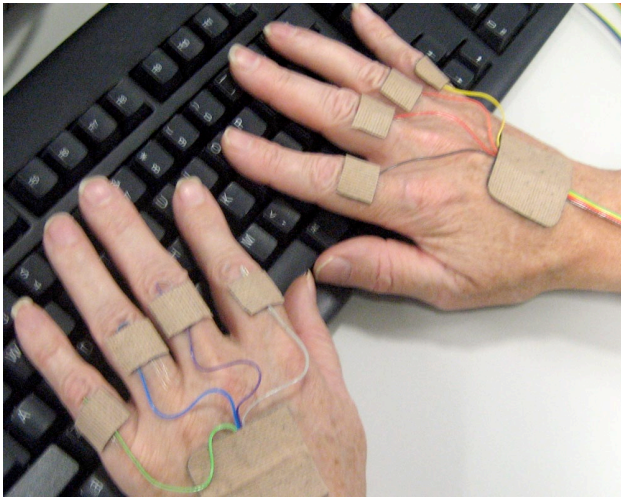
Figure 2: Electro-Tactile Interface comprised of Transcutaneous Electrodes fitted to the hands.
