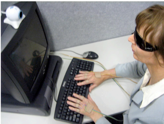
Figure 3: Hardware Components: Gaze-Tracking Spectacles/Camera and Electro-Tactile Interface
