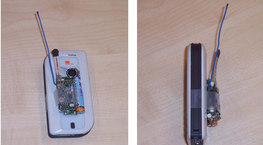
Figure 4.1: This figure shows a nokia series 60 mobile phone augmented with a Smart-It(Particle) on the backside. A designer can attach a Particle to the mobile phone in whatever position suitable. The Smart-Its board in pictures contains a 3D accelerometer, light sensor, temperature sensor, audio sensor, pressure sensor and a voltage sensor.
