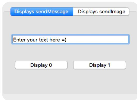
Enter a text in the textbox and press a button. A text will be sent to and drawn on the specified display.
