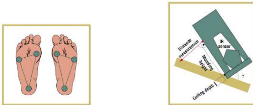
Figure 3.8: Force-sensor placement (left); IR-sensor setup (right)
