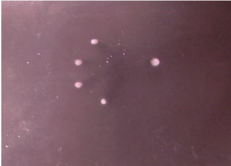
**Figure 2.4:** User touching the multi-touch surface as seen by an infrared-sensitive camera. All five touch points are clearly visible.
