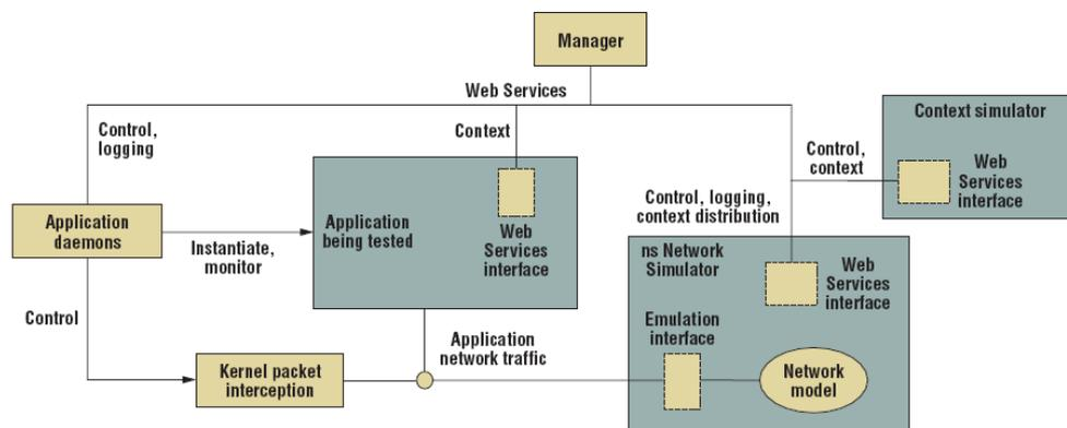
**Figure 2.6:** Setup of the evaluation system; The application code does not need to be changed after the web service interface was implemented
