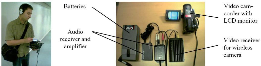
**Figure 2.1:** Data capturing for high quality data (cf. [Kjeldskov et al., 2004a])
