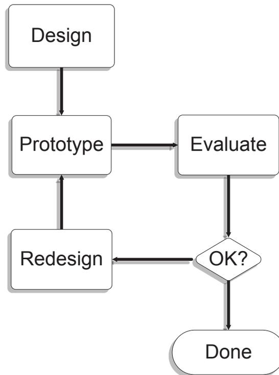
**Figure 1.4:** The iterative design process adapted from [DIX, 2003]
