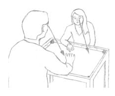
Figure 1. The envisioned GazeTop system: infrared (IR) cameras are placed at each corner of the table. IR LEDs are distributed around the perimeters of the table and act as point light sources. Multiple cameras, aware of the LEDs positions, observe the IR reflections on the user's eye and compute the gaze path [12]. This removes the need for a user calibration step. Unfortunately, a full discussion of this approach is outside the scope of this proposal.
