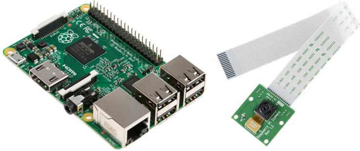
**Figure 3.1:** Left: Raspberry Pi 2. Right: Raspberry Pi camera module
