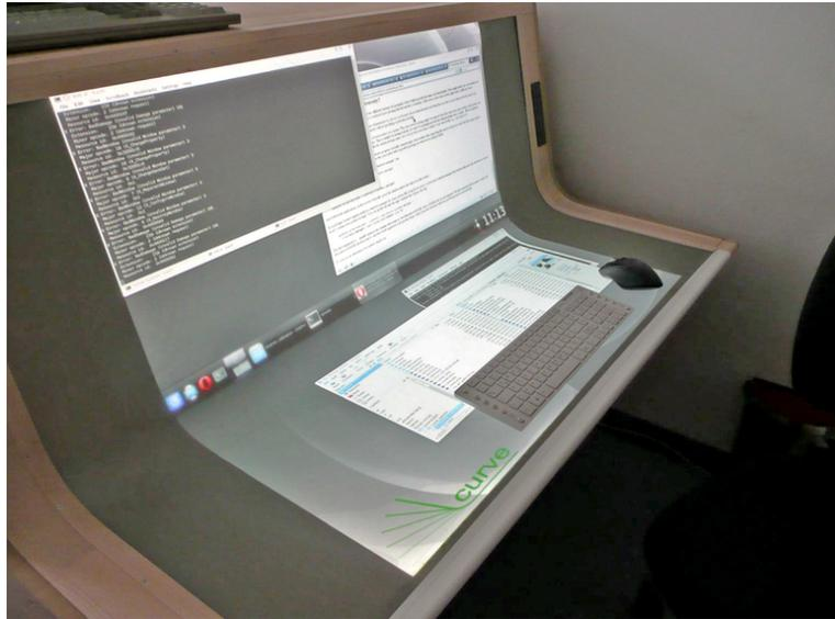
**Figure 2.1:** Curve is a digital desk concept that blends a horizontal and a vertical interactive surface (Wimmer et al. [2010])
