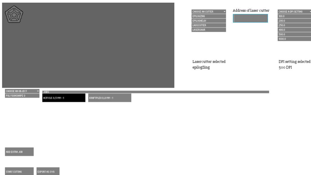
**Figure 3.9:** The Cut-Tool will open a dialog to send the created shapes to a lasercutter or export them as SVG-files
