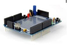
The MAKE Pack contains a kit for a <u>MakerShield</u> prototyping shield (see photo). **Solder** it together (URL for instructions on the pack), stick the mini breadboard onto it, and you have a very useful board with some built-in LEDs, buttons, even a
