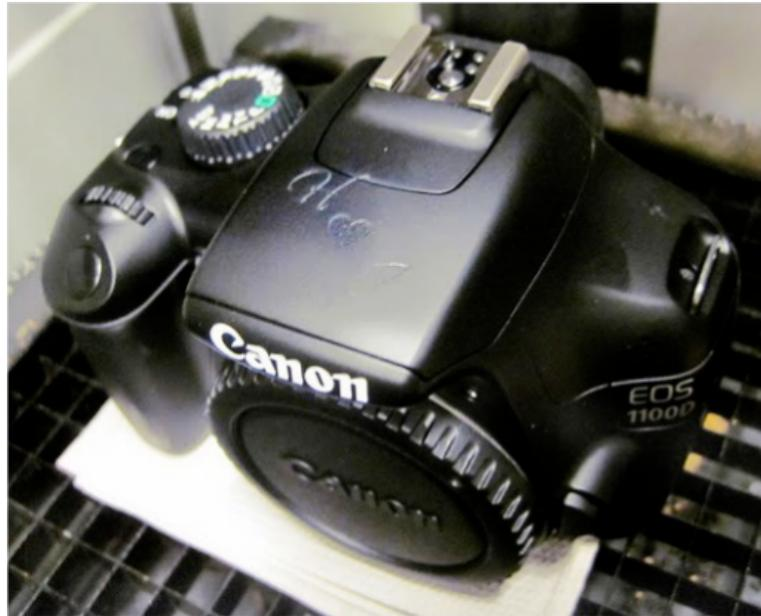
**Figure 1.5:** An expensive mistake: The engraving is not where it should be
