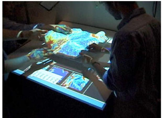
Figure 4. *Illuminating Clay*. The users are forming a landscape whereas the system projects additional information in real-time onto the clay [13].
