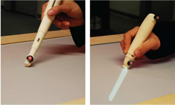
Figure 12. When pressing against the surface, the Beyond device collapses and is visually extended in the digital space. [10].
