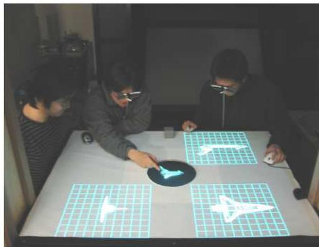
Figure 2. The IllusionHole system in use. The object in the center is perceived in 3D through the polarized glasses [12].
