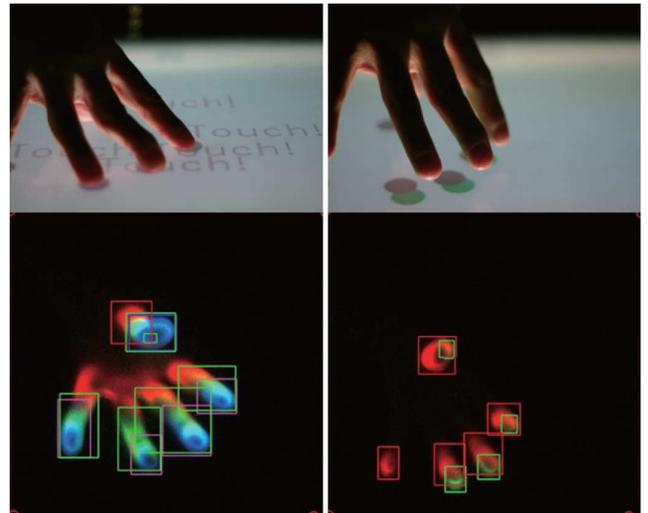
Figure 11. Touching vs. hovering. The position of a rectangle indicates where a blob has been detected. In this case the right hand is hovering over the surface [14].
