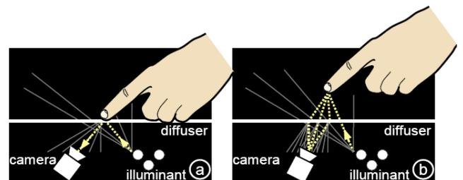
Figure 16. (a) Light is reflected with less scattering when the finger touches the surface. (b) Light is first scattered before it reaches the camera when the finger is above the surface [1].
