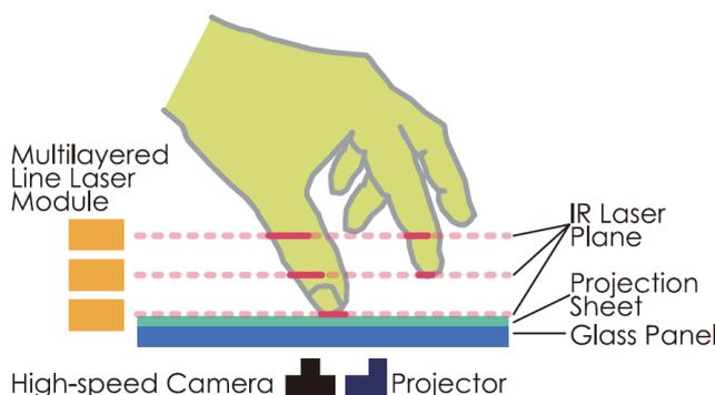
Figure 10. The Z-Touch configuration. Multiple line laser planes recognize finger angles by matching the detected distances at different heights [14].
