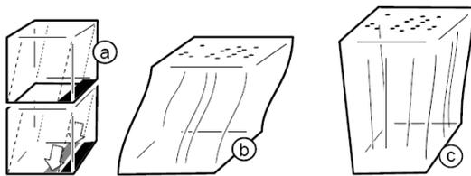
Figure 17. (a) The marker of the higher block is shifted. (b) Exemplified glass fiber bundle form for shifting. (c) Exemplified glass fiber bundle form for scaling down the markers [1].
