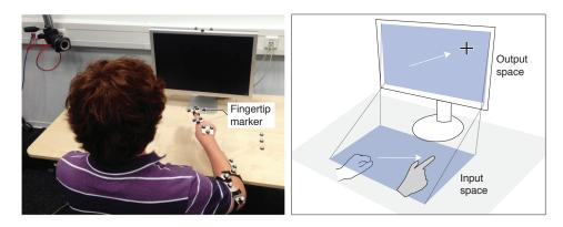
**Figure 4.4:** The hardware setup for our user studies (left), and the cursor mapping (right)<sup>1</sup>.
