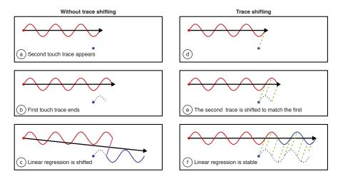
**Figure 2.12:** In (a–c), the interference of multi-touch traces that destabilizes the trajectory of the linear regression. In (d–f), the subsequent trace is shifted back, based on the offset of the first touch point in the new trace. (Modified image courtesy of [Kehrig, 2013])
