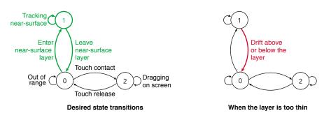
Figure 4.2: Left: A desired state model of near-surface input over a touch screen. Right: Input layers that are too thin cause the user to drift out of state 1.
