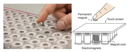
**Figure 5.2:** The FingerFlux prototype. An array of electromagnets, placed below a touch screen. Powering these electromagnets creates a magnetic force field that attracts or repels the permanent magnet at the fingertip. (Left image courtesy of [Weiss et al., 2011])
