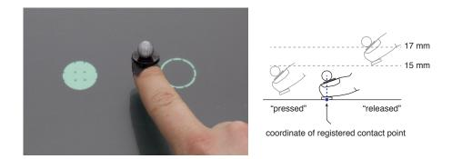
**Figure 5.4:** Hardware setup for the user study. Left: the marker setup. Right: The touch recognition thresholding. (Modified images from [Weiss et al., 2011].)
