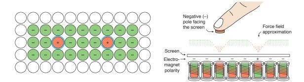
**Figure 5.3:** Left: A haptic feedback rendering scheme for two buttons (blue circles). Right: a cross-sectional view of the button row. The center of the buttons attracts the fingertip, while the area outside repulses. (Modified images from [Weiss et al., 2011].)
