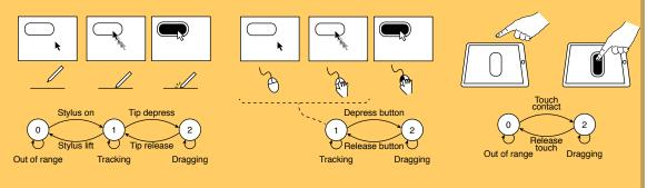
Figure 1.3: Input states of graphics tablet with a stylus, mouse, and touch screen
