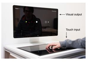
**Figure 3.2:** An indirect multi-touch system used in our experiments. (Modified image from [Voelker et al., 2013].)
