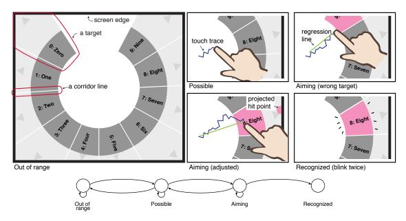
**Figure 2.8:** Visual guidance and feedback shown in each input state. Here, we illustrate a user intended to select "8:Eight", but initially aimed at "9:Nine".
