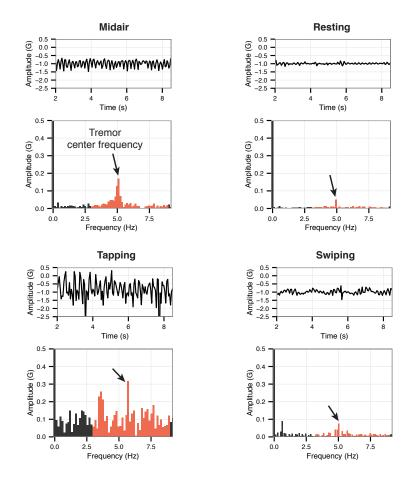
**Figure 2.4:** Examples of accelerometer data (top panels) and their Fourier transformation (bottom panels). The amplitudes in the tremor frequency range was increased by tapping, but swiping yields relatively low amplitudes. The frequency region we used in the analysis is highlighted. All data shown here were captured from the same participant (moderate tremor).
