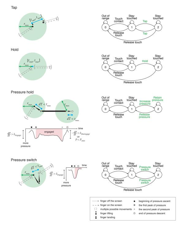
**Figure 3.4:** Interaction design schematic and state transitions of the four techniques. (Modified image from [Voelker et al., 2013].)
