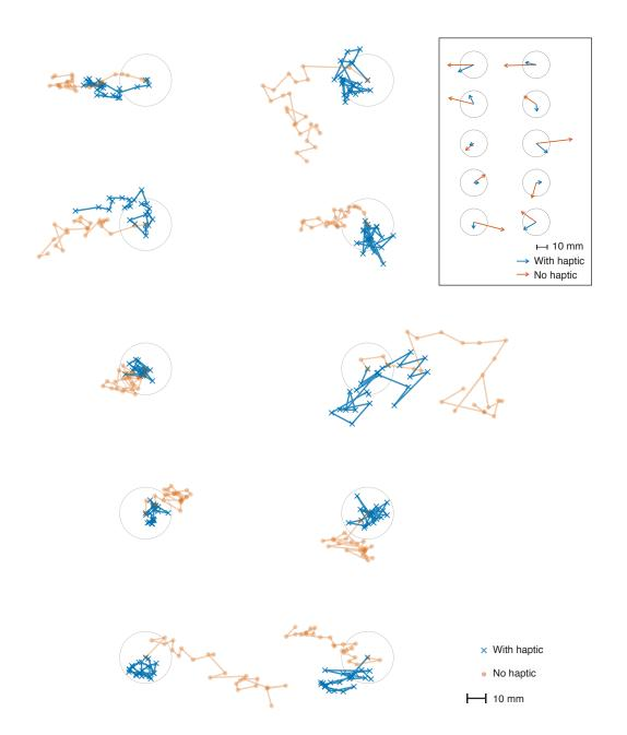
**Figure 5.5:** Contact points from each of the ten participants. The haptic feedback apparently reduces drifts. Only left targets were shown. Subsequent trials are connected with a line. The circle represents the button that is visible to the participants. The first trial always started at the center of the button. The inset shows the average direction and distance of these contact points.
