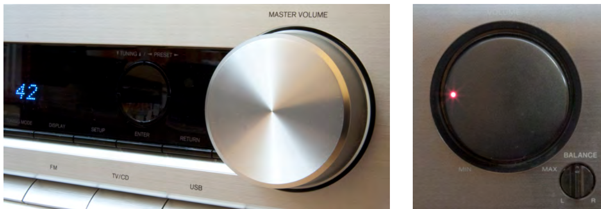
Figure 4.3: Volume knobs of HiFi audio receivers. Left: Infinite knob that changes volume relatively to the current value. It does not block at volume ranges and is easy to implement. However, an extra display is required to show the current volume. Right: Absolute knob with embedded analog volume indicator. Users can employ haptic memory to set a value. However, a motor is required to maintain digital-physical consistency when changing volume via remote control. Photos taken by the author.
