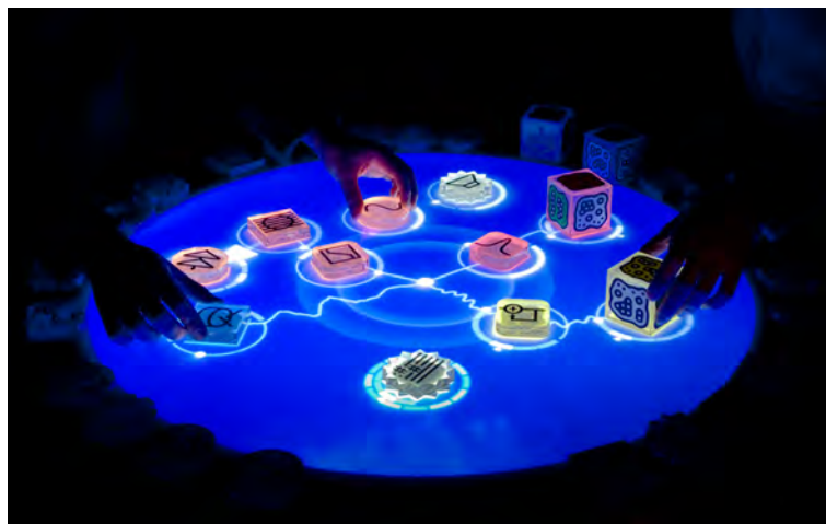
Figure 3.1: The reactTable is a musical instrument based on tangibles arranged on an interactive tabletop. Photo taken by Xavier Sivecas. Image courtesy of Jorda et al. [2007].
