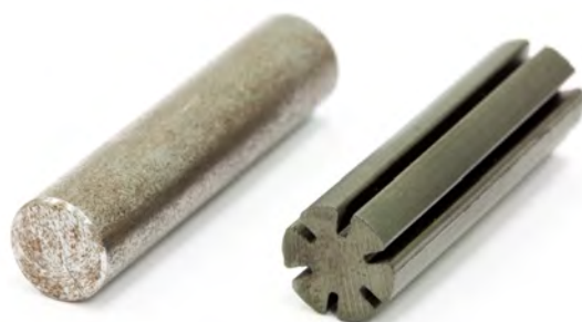
Figure 4.47: Different core materials. Left: Iron core. Right: Manganese-zinc ferrite core with recesses to avoid eddy currents.
