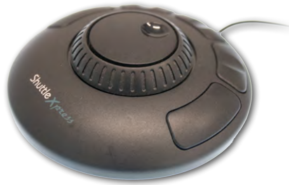
Figure 1.3: Input device for media navigation including two knobs and five buttons. A jog wheel in the center is surrounded by a spring-loaded knob that snaps back to its original position when released. Photo taken by the author.
