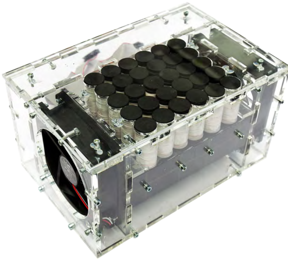
Figure 6.15: New FingerFlux table prototype containing 6 \times 5 electromagnets placed on a heat sink and cooled actively. Fingers are tracked using an optical tracking system.
