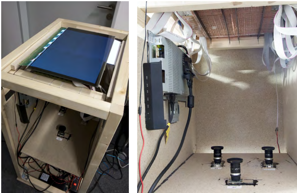
Figure 4.13: Implementation of Madgets Table. Left: The hardware is embedded into a wooden frame. Right: Cameras inside the table monitor the ends of fiber optical cables.
