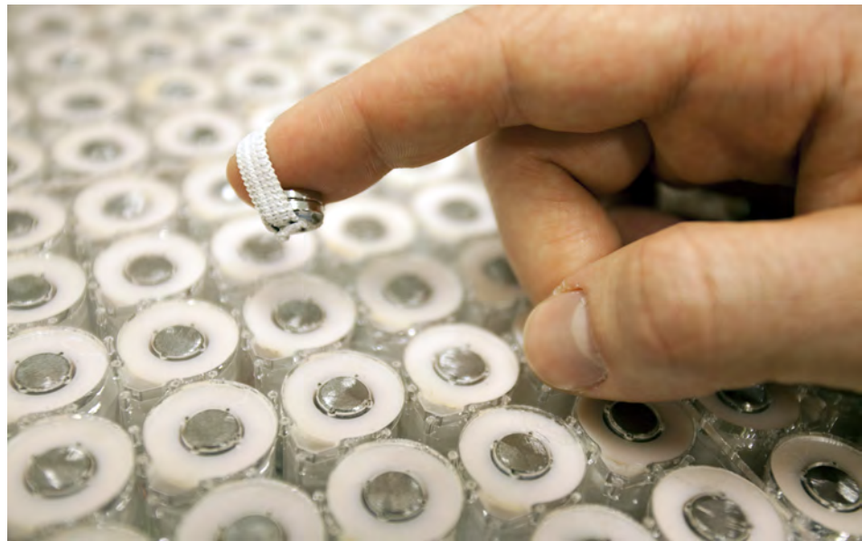
Figure 6.4: Concept behind FingerFlux. Electromagnetic fields reach well beyond the surface and apply forces to a permanent magnet that is attached to the user's finger. The permanent magnet passes these forces to the skin where they induce a haptic sensation. The table's backlighting and LCD display have been removed in this photo for illustration purposes.
