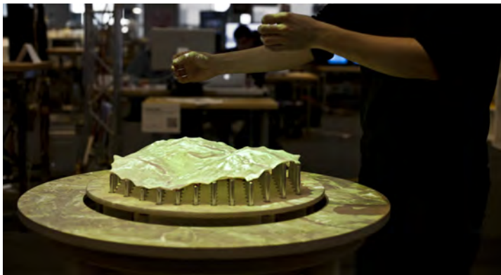
Figure 4.5: Relief contains 120 motorized pins that can generate height maps. Top projection on a Lycra surface provides a visual overlay. Users can perform input by pulling or pushing pins, by using external controllers, or via gestures above the surface by employing depth camera tracking. Image courtesy of Leithinger et al. [2011].
