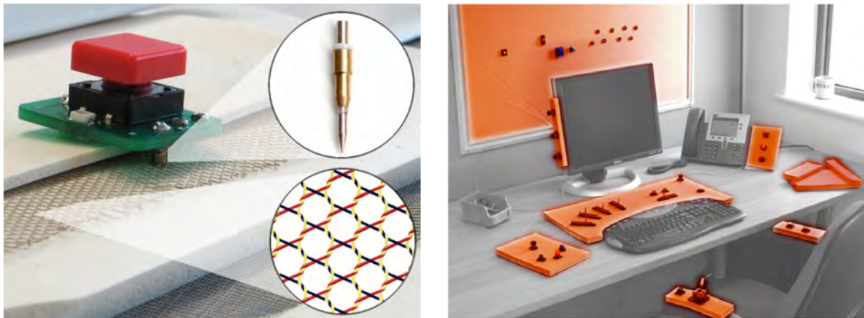
Figure 3.3: VoodooIO. Left: Technical principle. A control stuck into the surface closes a circuit and communicates its current state. Right: VoodooIO surfaces can extend a workspace in various ways. Image courtesy of Villar and Gellersen [2007].
