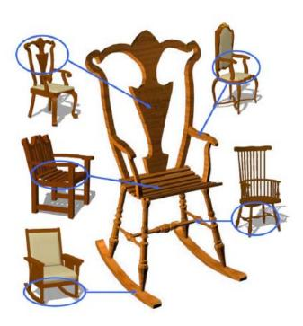
**Figure 2.13:** Modeling by Example: The chair in the middle is made up of the circled parts of the other chairs. In this method the model is composed of geometric parts extracted from a database of 3D models [FKS<sup>+</sup>04].
