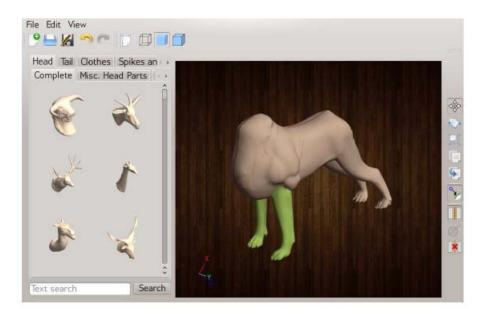
**Figure 2.14:** Assembly-Based Modeling: the model is made up of components in an intelligent list, which are extracted from a repository. Every time a component is added, the list is updated with the components which are related to the model [CKGK11]
