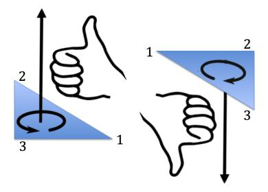
**Figure 2.2:** The right-hand rule defines the orientation of a triangle with the order of its points.
