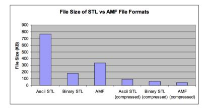
**Figure 2.3:** Size of STL and AFM formats in original and in compressed form [Hiller et al. 2009].
