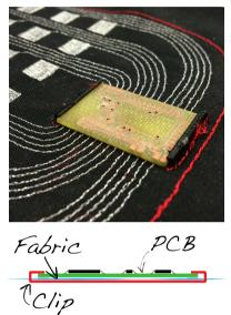
Figure 2: The connection between fabric (blue) and electronics is achieved by a clipping mechanism (red) that presses the ends of the conductive thread against conductive plates on the bottom side of the PCB (green).
