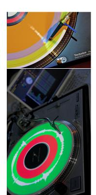
Figure 1: DiskPlay visualizes additional information directly on the timecode record of a digital vinyl system, integrating visual output and tangible controller in on device.
