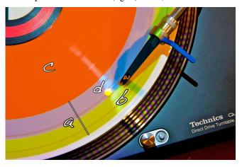
Figure 4. DiskPlay displaying a track. (a) Remaining playback area (blue). (b) Part already played as progress indicator (green). (c) Unused timecode part (red). (d) Cue points (yellow dots).
