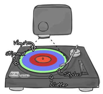
Figure 1. Using top projection, DiskPlay augments a white timecode vinyl disc with information about the structure of the current track, such as its starting point, length, and cue points.
