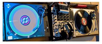
Figure 5. The DiskPlay test setup with the augmented turntable on the left and the traditional timecode vinyl on the right. The projector (not in the picture) is above the left turntable.
