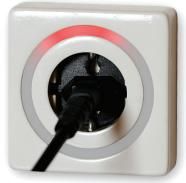
Figure 2. The PowerSocket showing low, medium, and high consumption levels.
