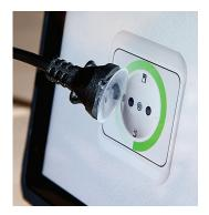
Figure 1. The software prototype of the PowerSocket. It combines the flexibility of a software prototype with simple hardware to simulate the physicality and "ambientness" of the envisioned product.
