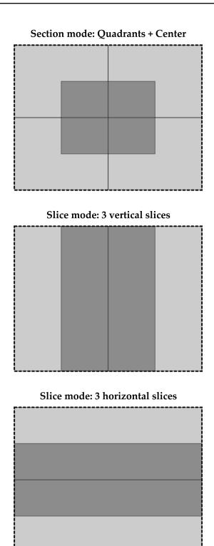
Figure 3.5: Detection for multiple QR codes
