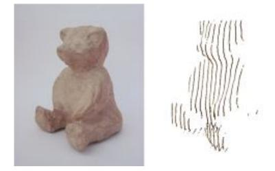
**Figure 3.3:** Scanning results from first prototype. Left: the physical object Bear. Right: the point-cloud of the Bear
