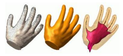
**Figure 2.7:** "Laser range data, the reconstructed watertight polygonal model, and its simplified medial axis." [AC01]
