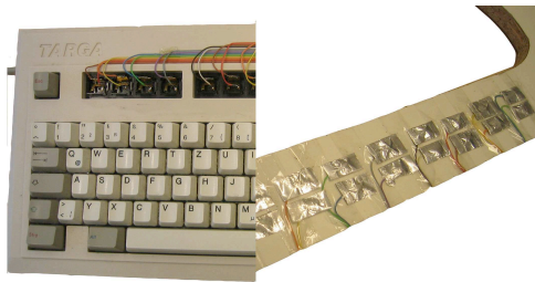
Figure 5: Each pair of contact surfaces is connected to a corresponding pair of contacts on the keyboard.
