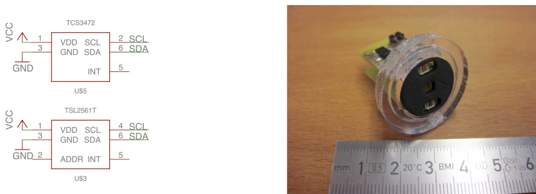
Figure 3.8: A photosensor with integrated evaluation circuit like the TCS3471 (RGB sensor) or TSL2561T (day light sensor) allows for higher resolution and easier evaluation
