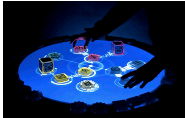
Figure 2.3: Reactable: A camera (orange) and a projector (blue) are mounted below the table. The camera tracks optical markers at the bottom of the tangibles, while the projector displays the screen image. Image source: http://mtg.upf.edu a
