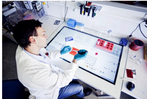
Figure 2.2: eLabBench: A camera (orange) above a screen (green) detects the position of probe racks. Additional information can be displayed on the desk. An infrared pen can be used for notes. Image source: http://www.version2.dk a
