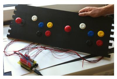
Figure 2.13: Arduino UNO attached to the game controller
