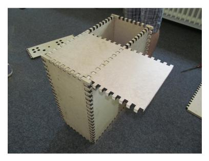
**Figure 2.2:** The Bottom part of the FabArcade. View from below, i.e. BOT H R is facing the top.
