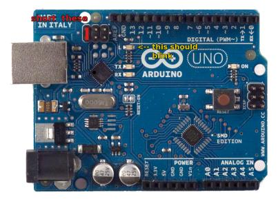
Figure 2.14: Short the shown PINs on the Arduino UNO
