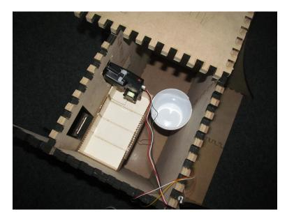
**Figure 2.4:** Bottom of the FabArcade from the inside. You can see the container for the money and the integrated coinslot. The wooden coloured, square box on the left is the container for the coins (white little bucket was just used while the glue dried to ensure the box does not fall down).
