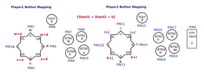
**Figure 2.15:** Key-to-button mappings for the game controller. The red letter denotes the key(s), which is reported to the host, while the blue PIN is connected to ground.
