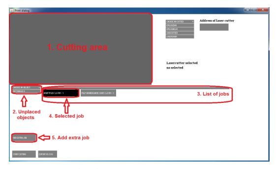
Figure 3.10: The interface of the cut dialog.
