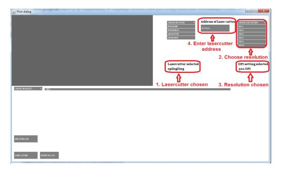
Figure 4.2: The settings which need to be set, after choosing a lasercutter type.
