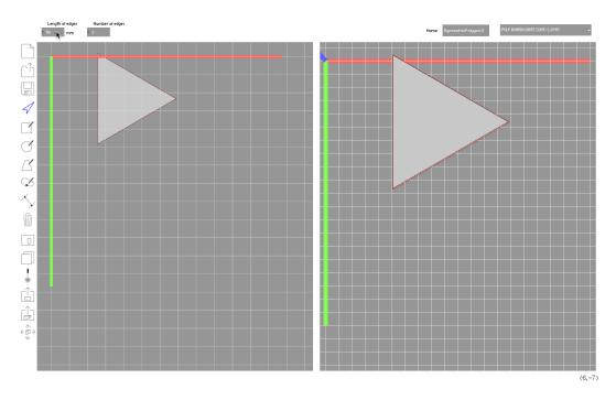
Figure 2.2: Changing the dimensions with the select tool
