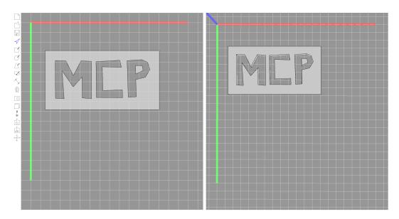
Figure 3.7: The Cutout-Tool can be used to add cutouts to existing shapes
