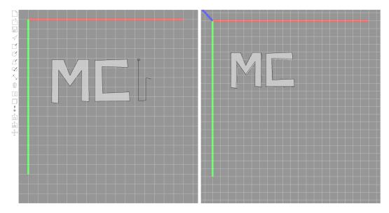
**Figure 3.4:** The "Draw Polygon"-Tool allows you to create custom shapes by simply drawing their outline.
