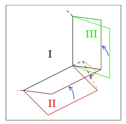
**Figure 5.5:** Use the perpendicular distance from intersection point and edge end point to the already connected edge to calculate the angle
