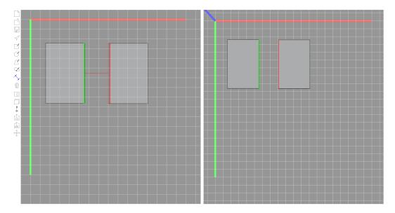
**Figure 3.5:** The Connect-Tool before the final click: The edge highlighted in green was selected first, the edge highlighted in red is the second edge to be selected
