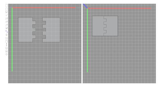
**Figure 3.6:** The Connect-Tool after the final click: Tenons for both edges have been created and the shapes were aligned.
