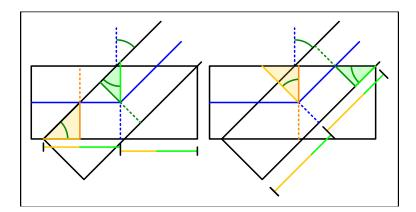
**Figure 5.1:** Triangle calculations to determine the outline dependent on angle between the shapes and their thicknesses
