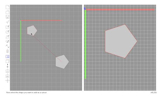
Figure 2.8: Add the smaller shape as a cut out to the bigger one
