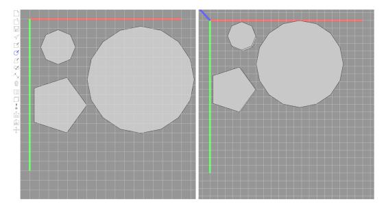
**Figure 3.2:** The "Draw Symmetric Polygon"-Tool can be used to create symmetric, concave polygons.
